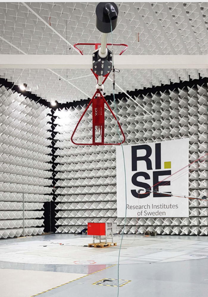
Inside the EMC test chamber (Awitar) at RISE in Sweden. Photo: RISE.
